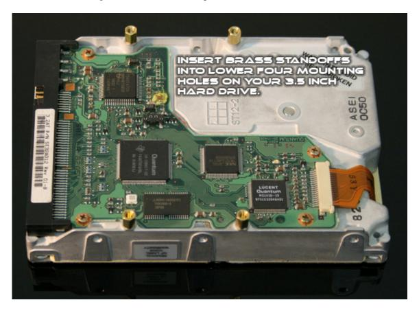
This will elevate the drive off the floor of the case allowing for better ventilation. Prop your partially assembled case up onto its back side and install the hard drive to the floor of the case using  $4 \times 10$ mm long 3m screws. The screws will go through the acrylic floor and fasten into the 4 brass standoffs on the hard drive. This time you can tighten the screws completely. The image on the next page shows you what this should look like.
