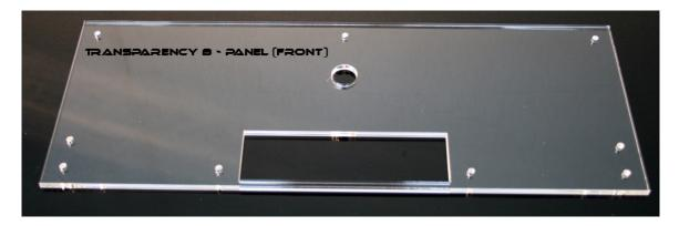
Next take 4 more 10mm long 3m screws and attach them to the blocks you just attached to the 'A' (bottom) panel. The long rectangular cutout orients down towards the floor of the case. This cutout is where your optical drive (cdr/dvdr) will interface with the case. Again do not fully tighten acrylic blocks – always leave slight play for future adjustment. Next locate panel 'C' and remove its wrap of film. The 'C' (rear) panel appears as illustrated on the next page:
