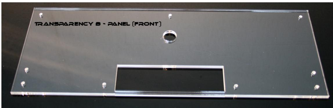
Next take 4 more 10mm long 3mm screws and attach them to the blocks you just attached to the 'A' (bottom) panel. The long rectangular cutout orients down towards the floor of the case. This cutout is where your optical drive (cdr/dvdr) will interface with the case. Again do not fully tighten acrylic blocks – always leave slight play for future adjustment. Next locate panel 'C' and remove its wrap or film. The 'C' (rear) panel appears as illustrated on the next page:
