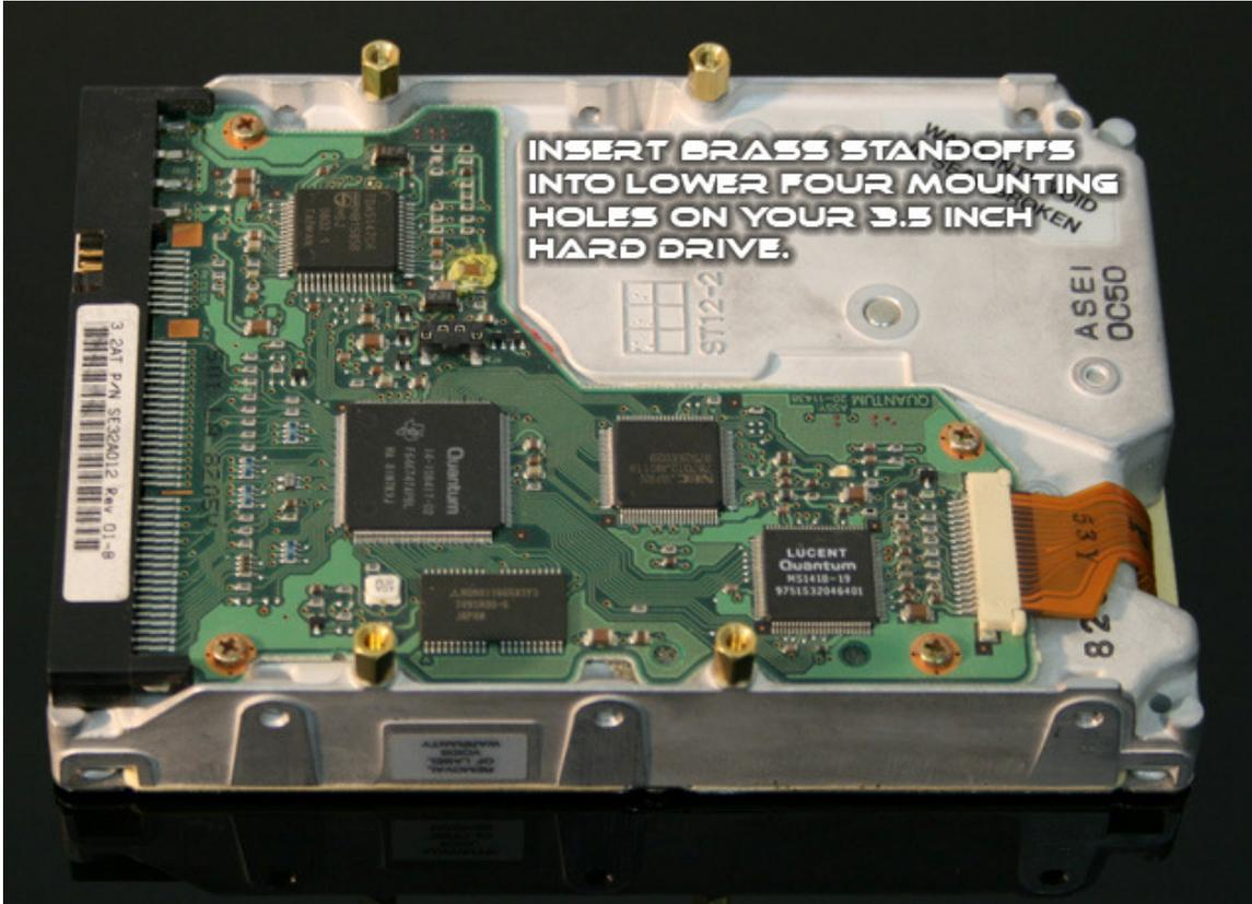
This will elevate the drive off the floor of the case allowing for better ventilation. Prop your partially assembled case up onto its back side and install the hard drive to the floor of the case using 4 x 10mm long 3m screws. The screws will go through the acrylic floor and fasten into the 4 brass standoffs on the hard drive. This time you can tighten the screws completely. The image on the next page shows you what this should look like.
