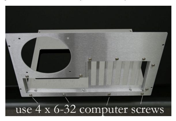
Now flip your 3 part assembly over (that's the I/O – Back panel – MB tray assembly). Place the assembly on the large flat surface area – where the motherboard assembles on the table. Allow for the Back Panel – I/O portion to hang down over the edge of the table. Use 3 x 6-32 computer screws to fasten into the I/O panel from the underside of the tray. This will tighten the assembly complete! See picture below for reference to 3 clearance holes/threaded inserts to fasten in this step.
